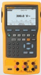
Fluke 754 Documenting Process Calibrator-HART See pg 23
